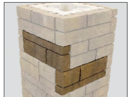
Diagram 25—Stagger veneers to break up lines
