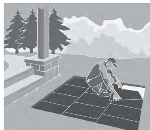
STEP 5: INSTALL EZ BASE PANELS
