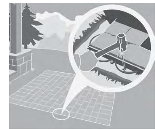
STEP 7: INSTALL EDGE RESTRAINTS
